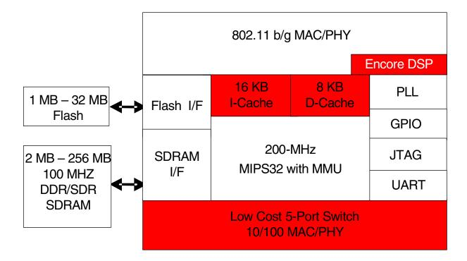
The BCM5352EL integrates a high-performance MIPS32 processor, IEEE 802.11 b/g MAC/PHY, SDRAM controller, and a configurable five-port Fast Ethernet (FE) switch.
